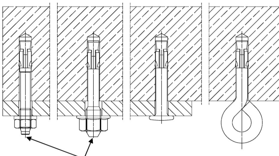
Additional marking only galvanised steel for  $h_{ef} = 25$  mm (centring, bar or points)
